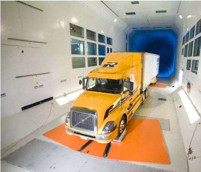
Figure 1: Volvo VN 660 and 28-ft. Trailer in the NRC 9m x 9m wind tunnel.
