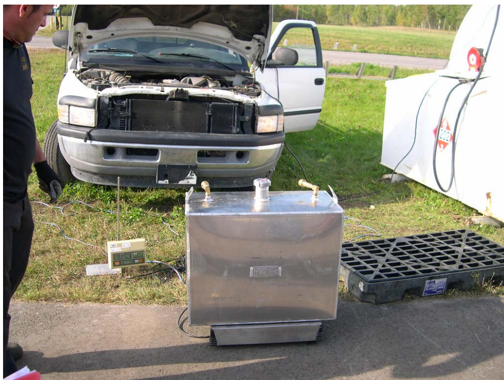
Figure 3. Temporary tank installation and weighing.
