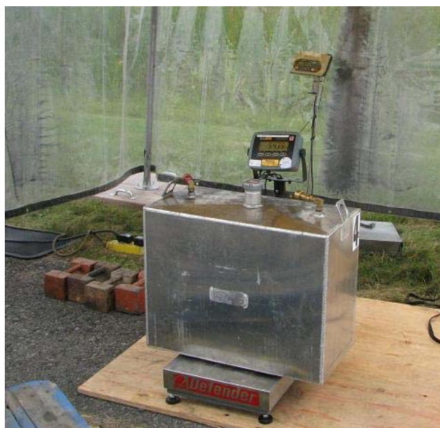
Figure 2. Installation and weighing of the temporary fuel tank.
