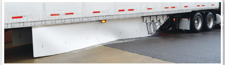
Above, the AeroFlex Composite completes drag testing by making 40 passes over a ramped loading dock. The composite panels can handle any typical impact situation and pop right back into perfect shape.
